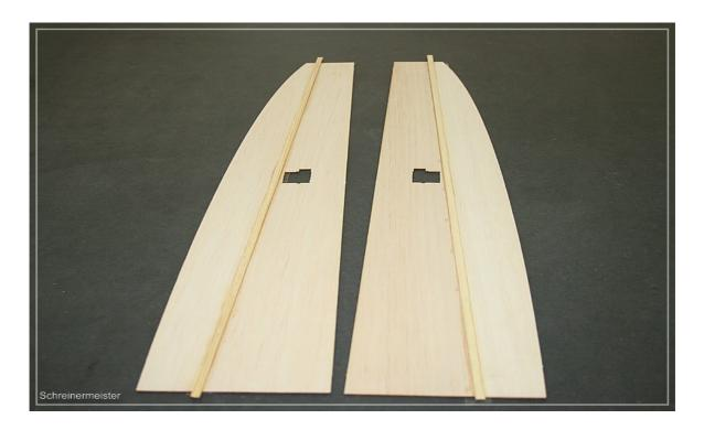
Then glue the spar to the skin by running cyano glue along the spar/balsa, while at the same time pushing it down on the skin. (A good trick is to use a screw top from a plastic-bottle as a finger protector. They are usually made of a material that does not stick to cyano, and you can push reasonably hard without having your fingers stuck to the wood.)
