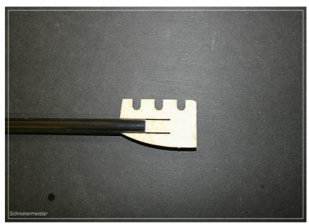
Now remove this part, leaving the cross in the tube. Next, make sure you have enough thin cyano. And be prepared for glue to run out of the carbon tube, so please, do not do this procedure on the living room carpet.
