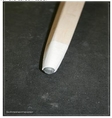
This allows you to sand the contours easily. Once you are happy with the results, soak the joints with cyano, to make sure it all sticks together properly. The carbon tube is NOT fitted yet!
