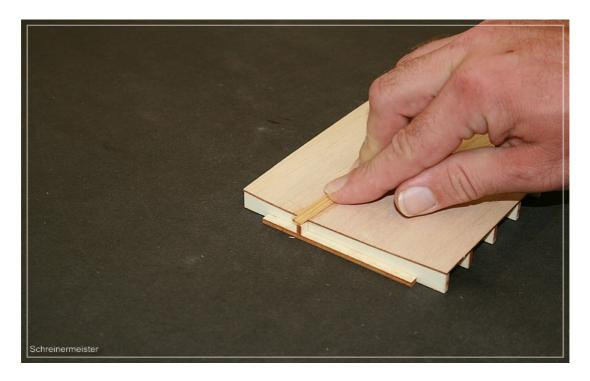
When the glue has dried you place the skin on the jig. You did not remove the sellotape yet did you? If you did, put it back (or better, put a fresh piece on the joint. To secure the skin in the jig, simply use a few small drops on the sellotape to stick it temporarily to the jig. Don't overdo it, you simply only want to stick it to the sellotape, not the wood!!
